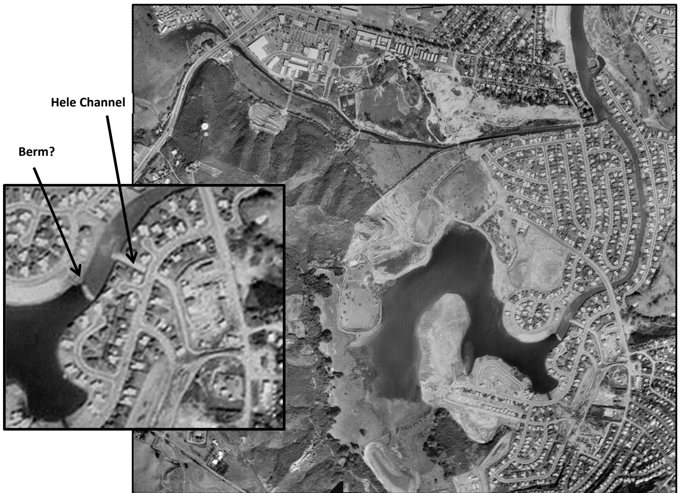
Figure 6. 1963 aerial photo of Enchanted Lake under construction. Note lack of Kawainui levee and presence of berm across stream exit from pond with heavy silt load entering from Hele Channel inlet (enlarged inset) where the stream channel is still very shallow. USGS: EKM-2CC-246, 1-14-63.
