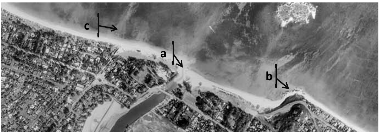
Figure 29 1963 aerial (USGS EKM-2CC-246) dated 1-14-63 prior to construction of Kawainui Levee. Note stream flowing across sand beach (a), and wide sand beach continuous around Aala Point and into Lanikai (b). Location of historic stream mouth channel (~1850 nautical chart) can be seen ~1,000 feet to the west (c).
